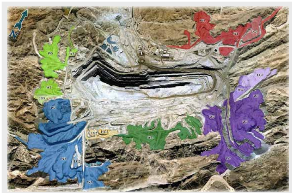
Figure 2: Location of rock dumps relative to the open pit. W (waste rock), LG (low-grade stockpiles) and HG (high-grade, high calc stockpile).
